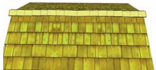
**61.** Place 3rd Ridge Cap 8" back from 2nd (enough to cover shingle nails). Attach 3rd Ridge Cap as per **Step 60**. Continue to position and attach Ridge Caps until half the roof is complete. From opposite side, position and attach Ridge Caps as described above. Score/cut 1 Ridge Cap to 12" or to fit in the center of roof. Attach center cap with **4 - 1 1/2" Shingle Nails**.
