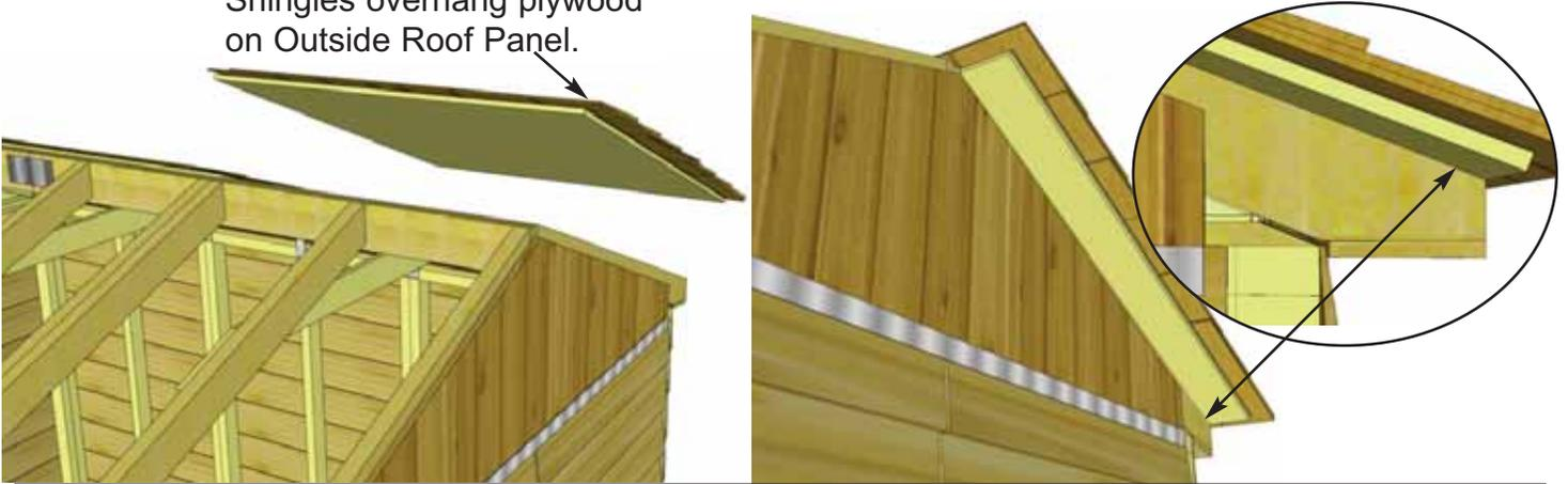
**41.** Lift up, position and attach 2nd **Outside Roof Panel** on Rafters as per **Step 39**.
