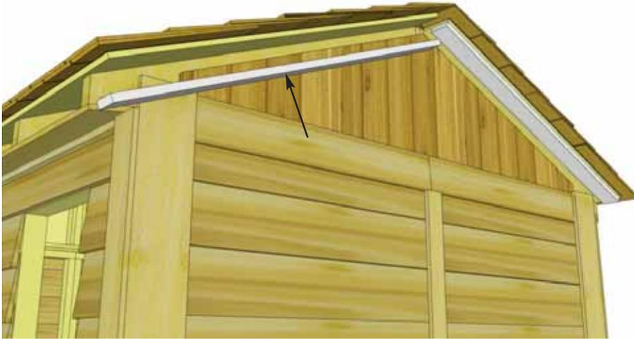
**56.** Attach **Facia Nailing Strips** to the underside edge of the plywood roof. Align corner of Nailing Strip with corner of roof plywood. Secure each Strip with **3 - 1 1/4" Screws**. Complete all four pieces, two on each side of the shed.
