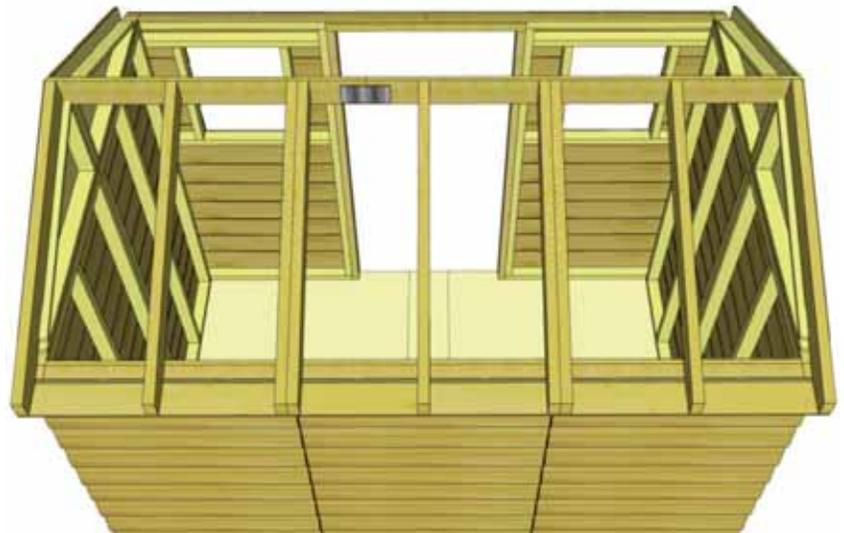
**31.** When Rafter Section is correctly positioned, outside rafters will sit equally on gable framing and Soffit will sit approximately 1/8" away from wall panels.
