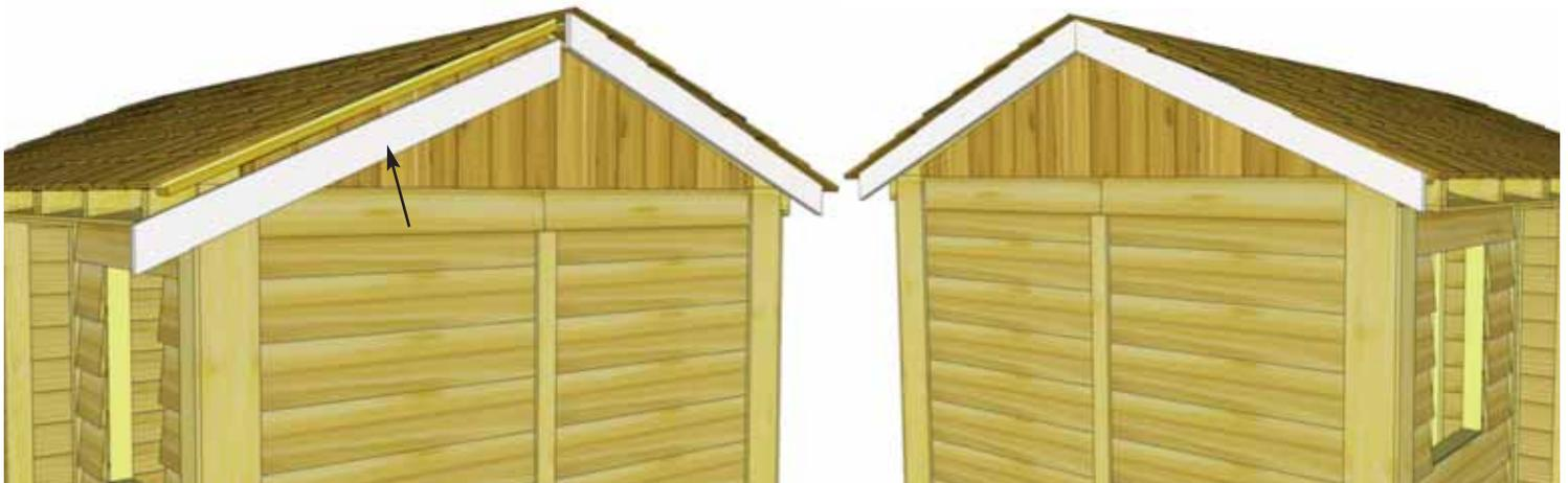
**57.** Attach **Side Facia** to end of roof panel plywood and Nailing Strip. Line Facia up to form a peak and attach to Nailing Strip/plywood with **6 - 1 1/2" Finishing Nails** per piece. End of Facia should be aligned flush with end of Rafter. See **Step 58** for detail. Gap where Facia boards come together at peak will be covered in **Step 59**.
