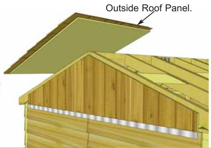
**38.** Identify all Roof Panels. There are 4 Outside and 2 Middle Roof Panels. Outside Panels will have shingles overhanging the plywood on one end. Lift up and place an Outside Roof Panel on Rear Rafters.
