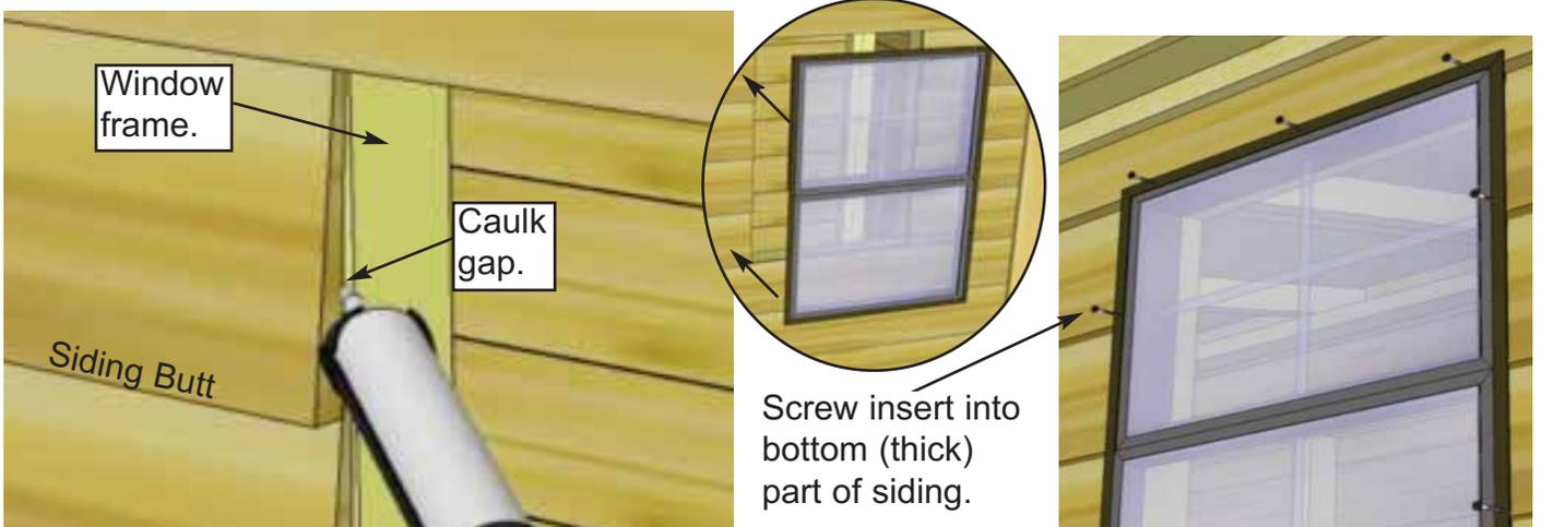
**70.** To reduce possible water from penetrating into the window cavity, caulk gap on both sides of window opening prior to installing **Window Insert**. Position insert in cavity and screw with **6 - 1 1/4" Screws**. On sides, make sure to screw insert into the thick butt of the siding only.
