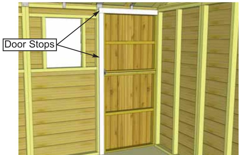
**D.** Attach 1 Vertical and Horizontal Door Stop. See **Step 69** for detail. You may have to trim Horizontal Door Stop to fit.
