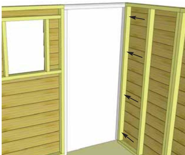
**C.** When correctly aligned, attach Door Jamb to wall stud with **4 - 2 1/2" Screws**.
