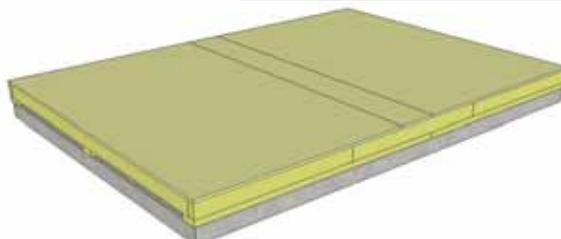
**Important - Make sure floor is level before moving on to wall section. Use a level to confirm, and shim floor joists as required.**
