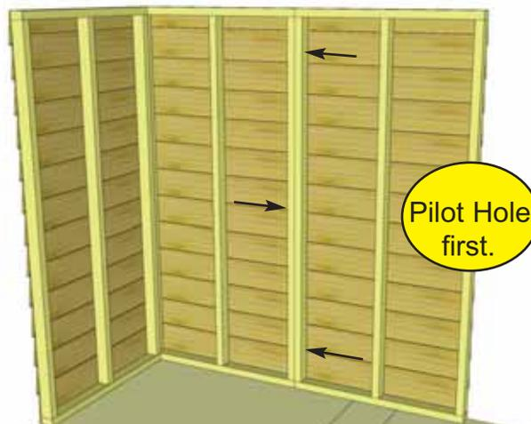
**14.** Position and attach 2nd rear wall panel as shown above. Attach adjacent wall studs together with **3 - 2 1/2" Screws**.
