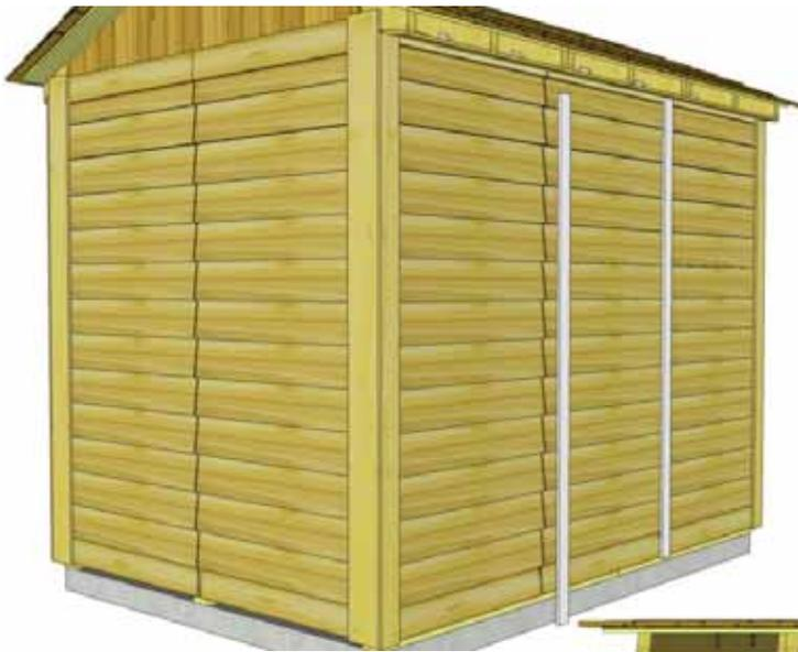
**54.** Attach **Rear Wall Narrow Trim** where wall panels come together and leave a seam. Position trim equally on wall seam and tight underneath Soffit and Rafter. Use **8 - 1 1/2" Finishing Nails** per piece to secure.
