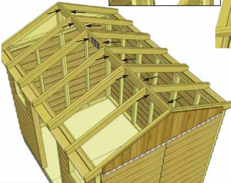
**33.** At the peak, align Ridge Boards so they are flush together and secure them with **12 - 1 1/4" Screws.**
