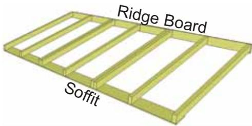
**29.** Flip Rafter Section over so Soffit is facing down. Starting with the rear Section, lift completed rafters up and place on gable framing.
