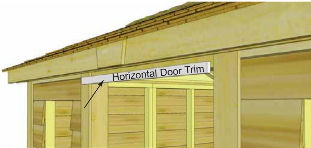
**63.** Attach **Horizontal Door Trim** with **4 - 1 1/2" Finishing Nails** to cover Door Header.
