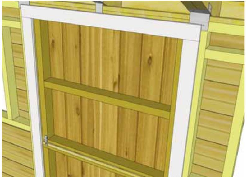
**69.** Attach Interior Door Stops to door framing (Jambs and Header). Start with **Vertical Door Stops**. Stops should overlap doorway by 1/2". Use **4 - 1 1/4" Screws** to secure each piece. Attach **Horizontal Door Stop** next using **3 - 1 1/4" Screws**.
