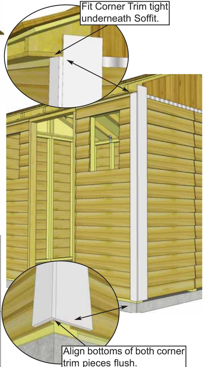
Fit Corner Trim tight underneath Soffit.
