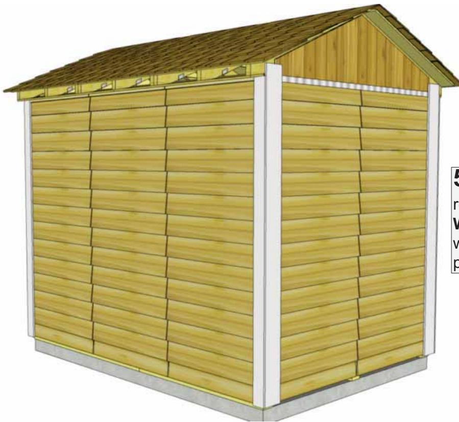
**52.** Trim out rear corners with remaining pieces of **Corner Trim** and **Wide Corner Trim**. Align and attach with **8 - 1 1/2" Finishing Nails** per piece as per **Step 51**.
